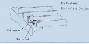
place. Welding of the grating panel to the supporting members provides the most rigid, permanent installation. Where panels may have to be removed, the F-9 saddle clip fastener is recommended for most mezzanine installations. A nut and bolt, stud or
